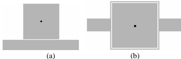
Fig. 2. (a) Microstrip loaded with the ground patch resonator, (b) Proposed resonator: grounded patch embedded in the microstrip.
