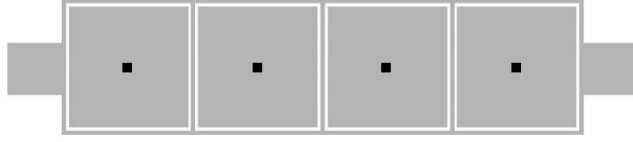
Fig. 4. Layout of the proposed stopband filter of the fourth order.
